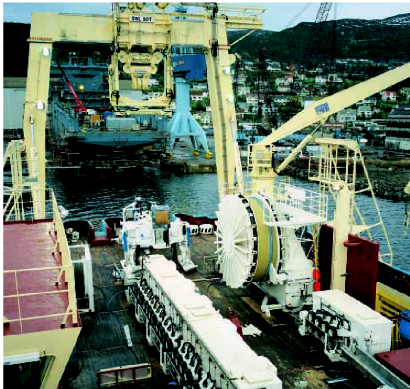
Figure 9. Typical cable repair vessel fantail showing a high capacity A-frame (in this case, 60 ton SWL), a linear cable engine at center, and a 3 m diameter cable drum on the port side. The large, open deck is adaptable to a wide range of heavy lift operations.
