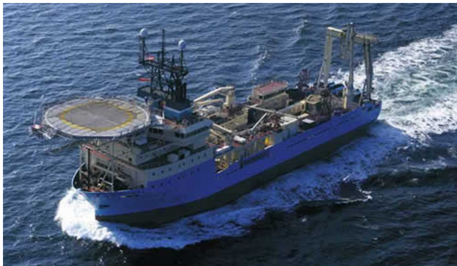
Figure 8. Global Marine Systems cable lay/repair vessel Maersk Recorder . The ship is 106 m LOA and has twin screw main propulsion, twin stern tunnel thrusters, a bow tunnel thruster, and a steerable bow thruster. The ship is equipped with a stern A-frame rated at 60 ton SWL, a 60 ton SWL tow winch, and a range of heavy lift tackle rated at 35-45 tons SWL.
