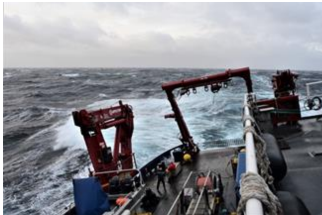
Waverider mooring deployment. Photos UW APL.
