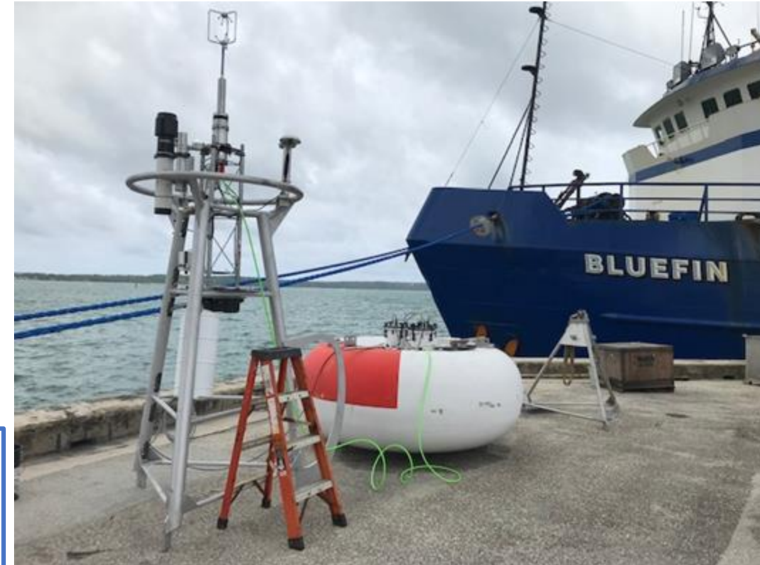
On the NOAA OCS Papa mooring, the WHOI DCFS would be placed on ring as a secondary wind system
