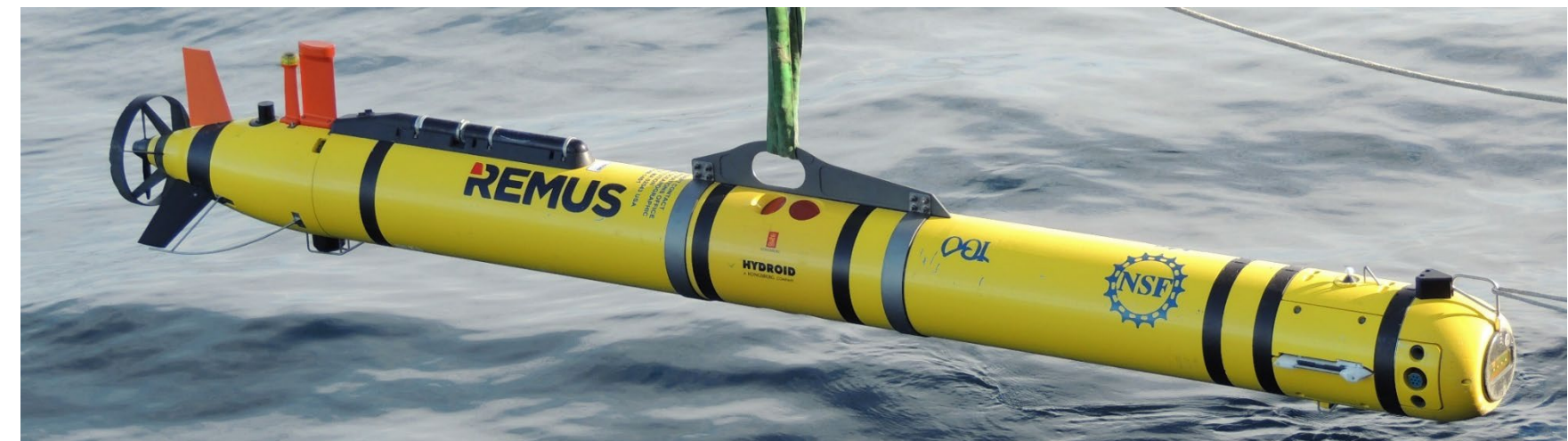
AUV CTD, oxygen, fluorometer, PAR, ADCP, nitrate
