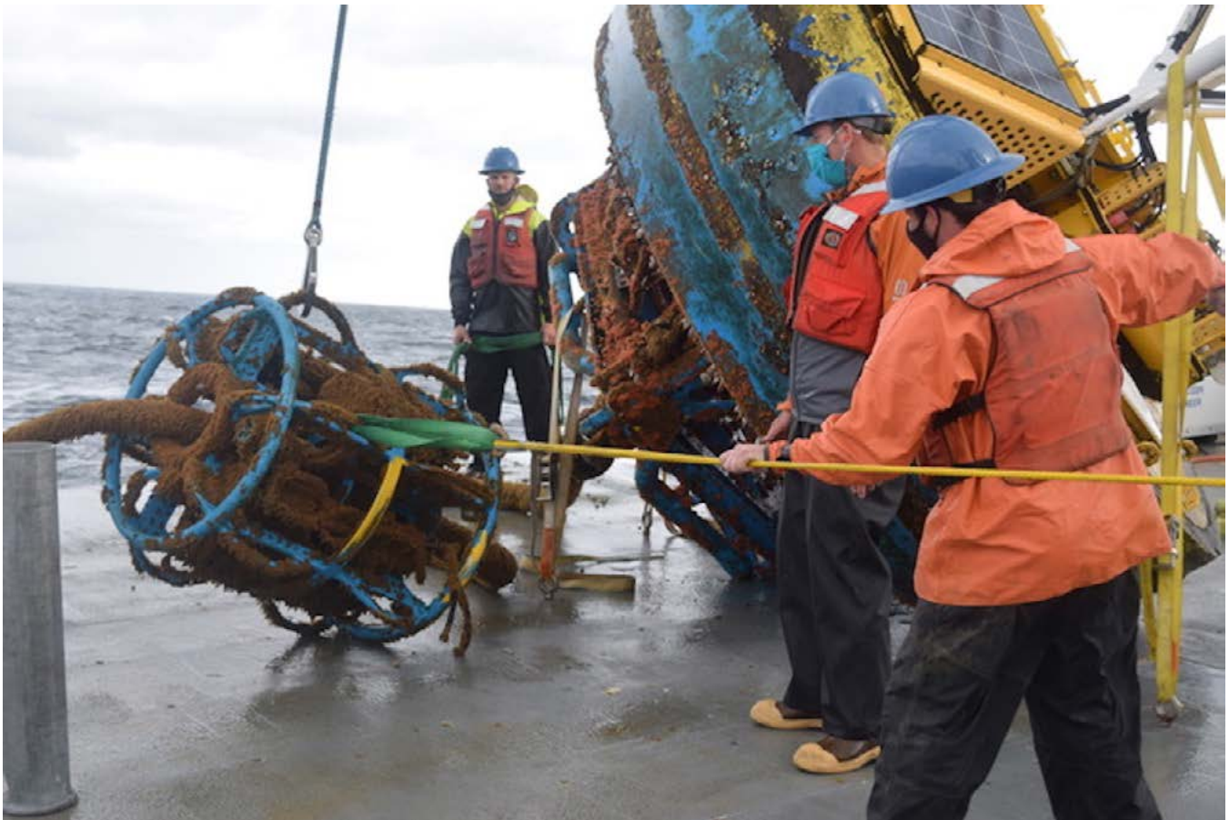
FIGURE 2.12 The Pioneer Team recovers the Inshore Surface Mooring after deployment in the water for 12 months. Credit: Dee Emrich, Woods Hole Oceanographic Institution.
