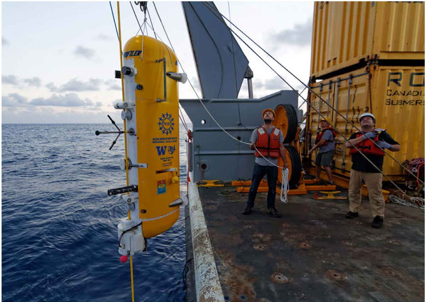
FIGURE A. A Regional Cabled Array instrumented Deep Profiler deployed off the fan tail of R/V Thomas G. Thompson during the 85-day 2014 installation cruise led by Chief Scientist John R. Delaney, University of Washington. Credit: M. Elend, University of Washington, V14.
