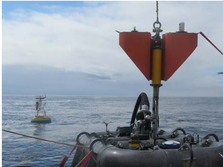
FIGURE 5.6 Lowering release lifting a mooring's Multi-Function Node.. Credit: Jonathan Fram, Oregon State University.
