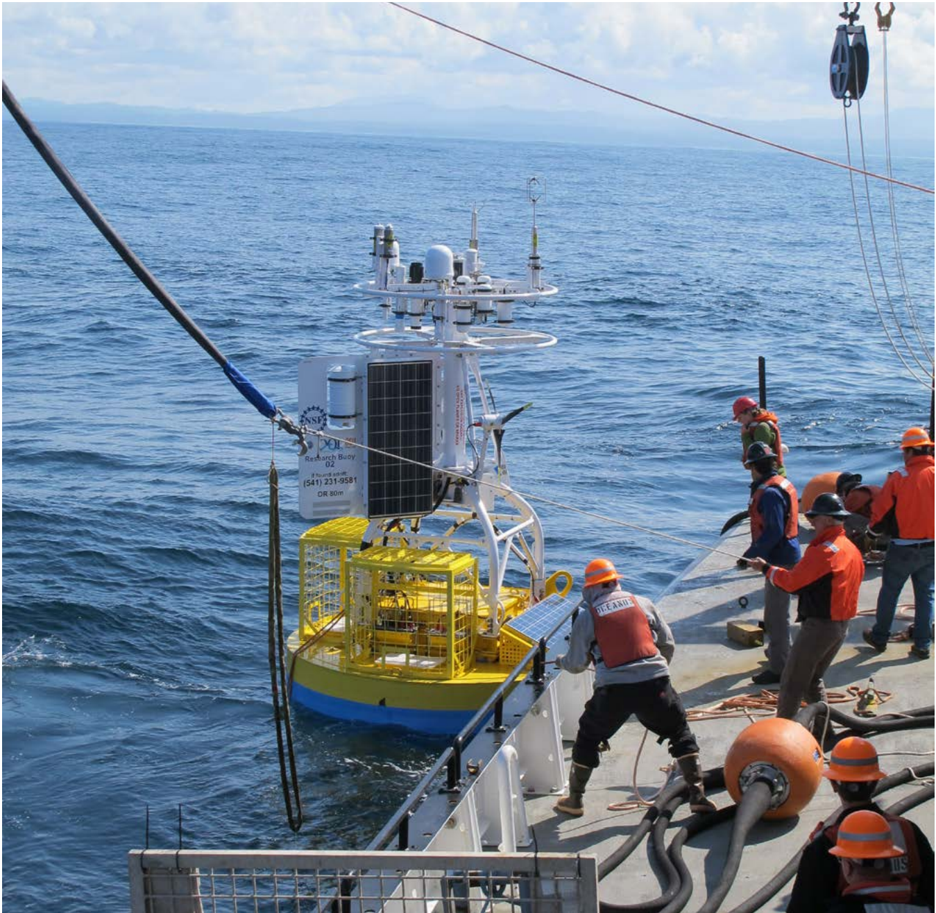
FIGURE 4.2 The Oregon shelf surface mooring is released from the crane by EA science party field chief, Walt Waldorf. Credit: OOI Endurance Array Program, Oregon State University.
