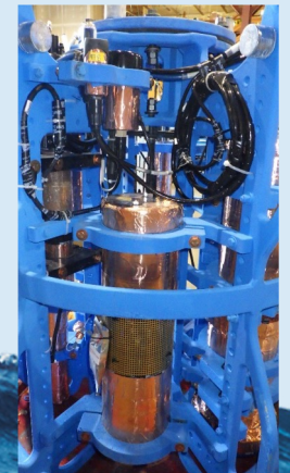
SAMI-pH sensor installed in the 7 m instrument frame (NSIF)
