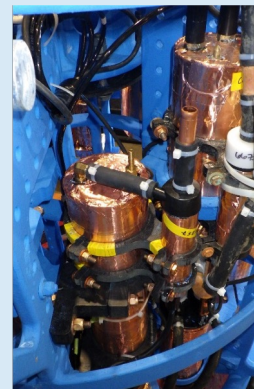
CO 2 -Pro CV mounted on the 7 m platform (Near-Surface Instrument Frame, NSIF) showing intake plumbing and exhaust.
