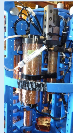
Deep SeapHOx installed in the 7 m instrument frame (NSIF)
