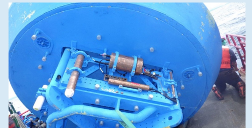
CO 2 -Pro ATM on the subsurface instrument plate just above the SBE 37 CT sensor. Water intake is at 1 m nominal depth.
