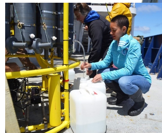
CTD is deployed off the R/V Revelle during the Visions '18 cruise, RCA shallow profiler, and an undergraduate student performing sampling. Credits: M. Elend, UW
