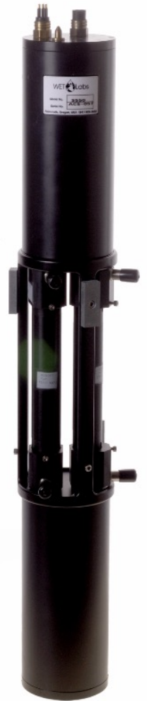
WET Labs' ac-s in-situ spectrophotometer provides simultaneous beam attenuation and absorption coefficients at four nanometer resolution across the visible spectrum. (Photo Courtesy of WET Labs)
