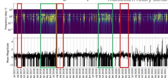
Above: Bubble activity in sonar backscatter, with red boxes indicating constant venting and green boxes indicating weak, intermittent venting. Upper panel shows frequency spectrum with white dashed lines at tidal periods. Bottom panel shows dimensionless backscatter intensity. (Marcon et al., 2022)
