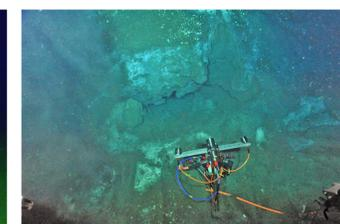
Above: Camera at in front of Einstein's Grotto, imaging individual bubbles escaping the vent which is in view of the bubble sonar.
