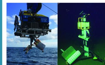
Above: Cabled R2Sonic 350 kHz multibeam rotary sonar, during deployment with the ROV Jason. (Marcon et al., 2019)
