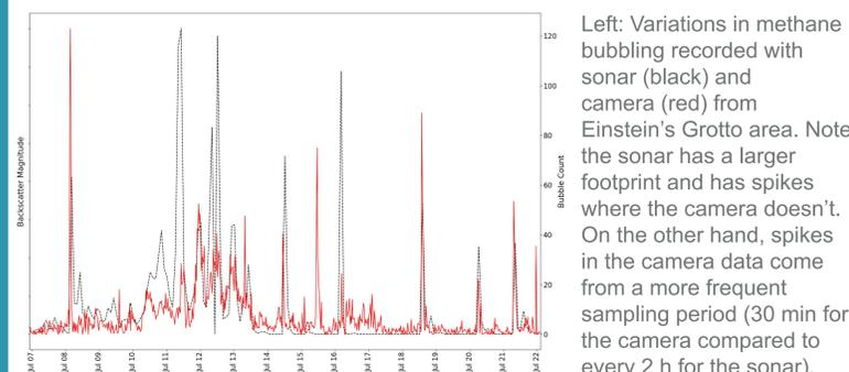
Left: Variations in methane bubbling recorded with sonar (black) and camera (red) from Einstein's Grotto area. Note the sonar has a larger footprint and has spikes where the camera doesn't. On the other hand, spikes in the camera data come from a more frequent sampling period (30 min for the camera compared to every 2 h for the sonar).
