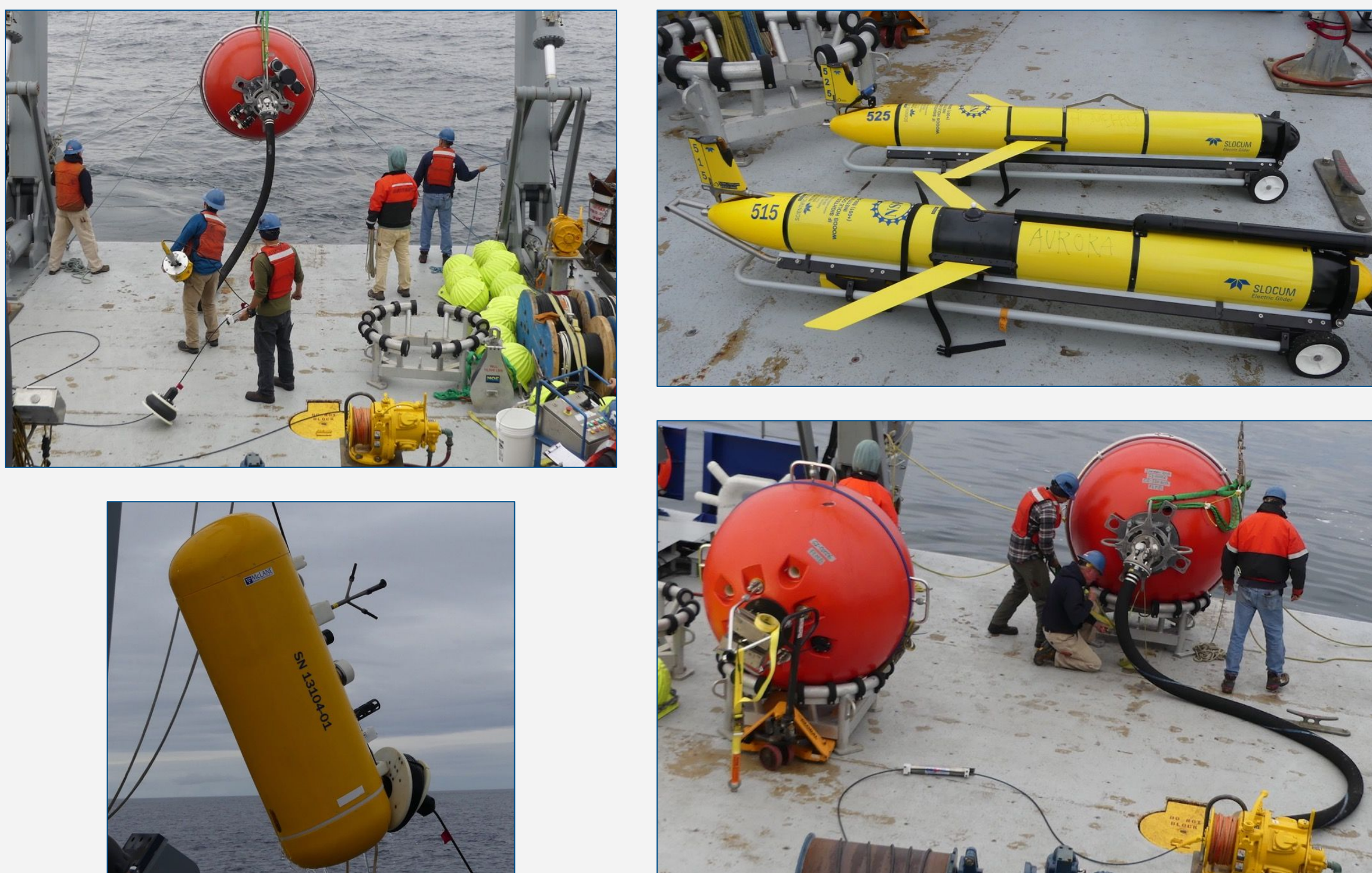
Figure 1 - Top: Schematic of a global array. Bottom (clockwise from top left): A global hybrid wire-following-profile mooring being deployed; two global open ocean gliders; a global surface mooring being deployed; a wire-following profiler.
