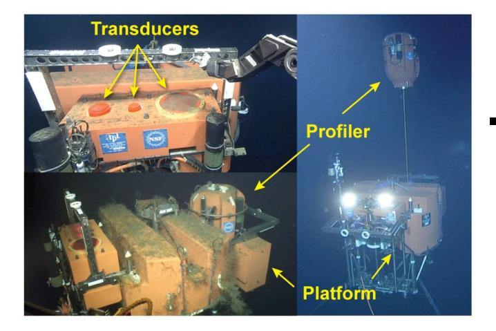
The echosounder contains 3 transducers transmitting at 38 kHz, 120 kHz, and 200 kHz
