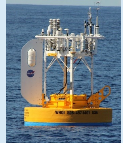
Addition of infrared hygrometer for moisture fluxes and thereby latent and sensible heat fluxes
