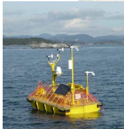
WindSentinel Metocean buoy (from Dominion SAP)
