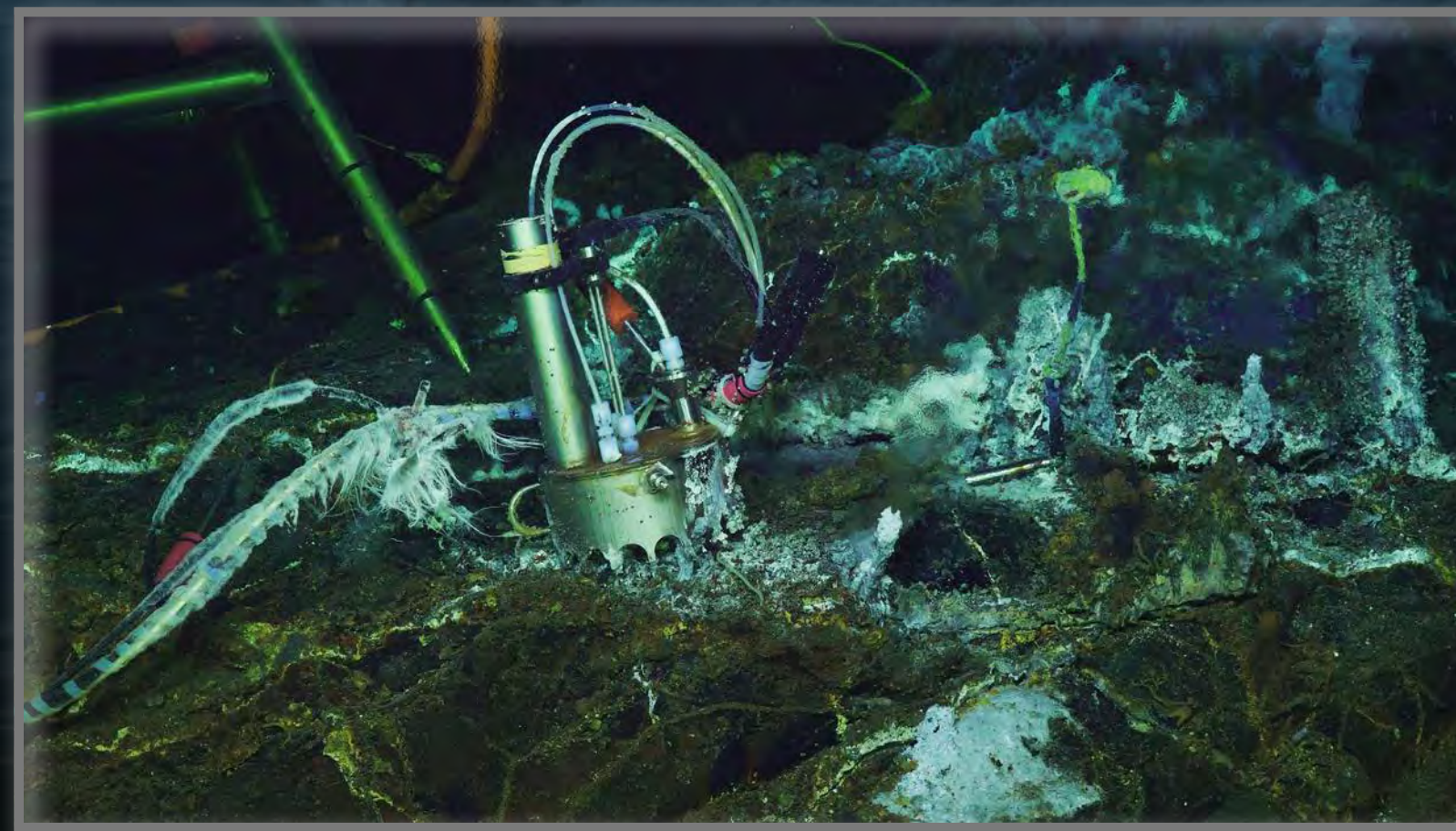
Vent cap with inlets to RAS-PPS
