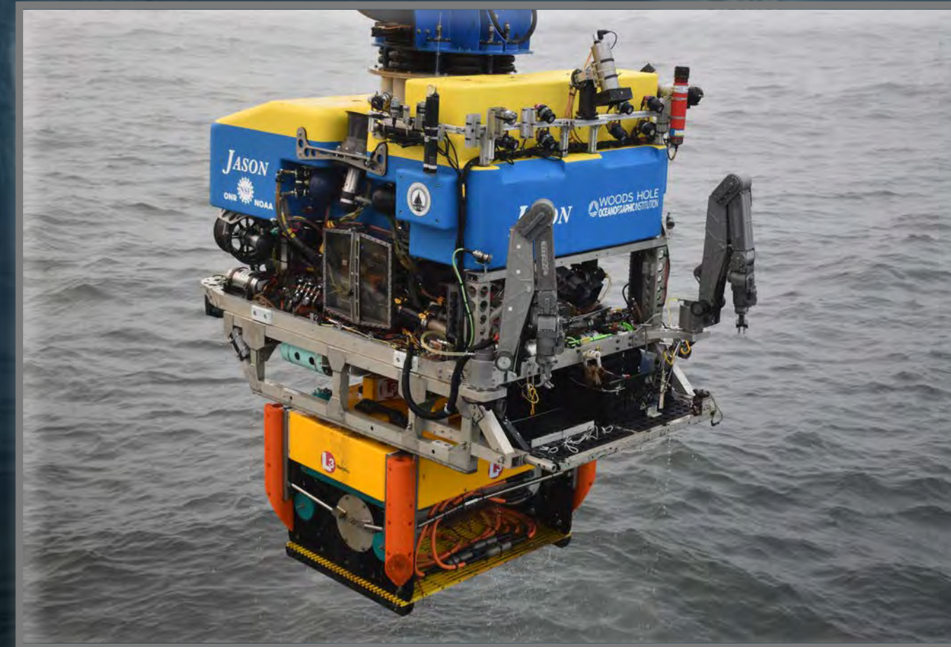
Science Interface Assembly Recovered onto the TGT
