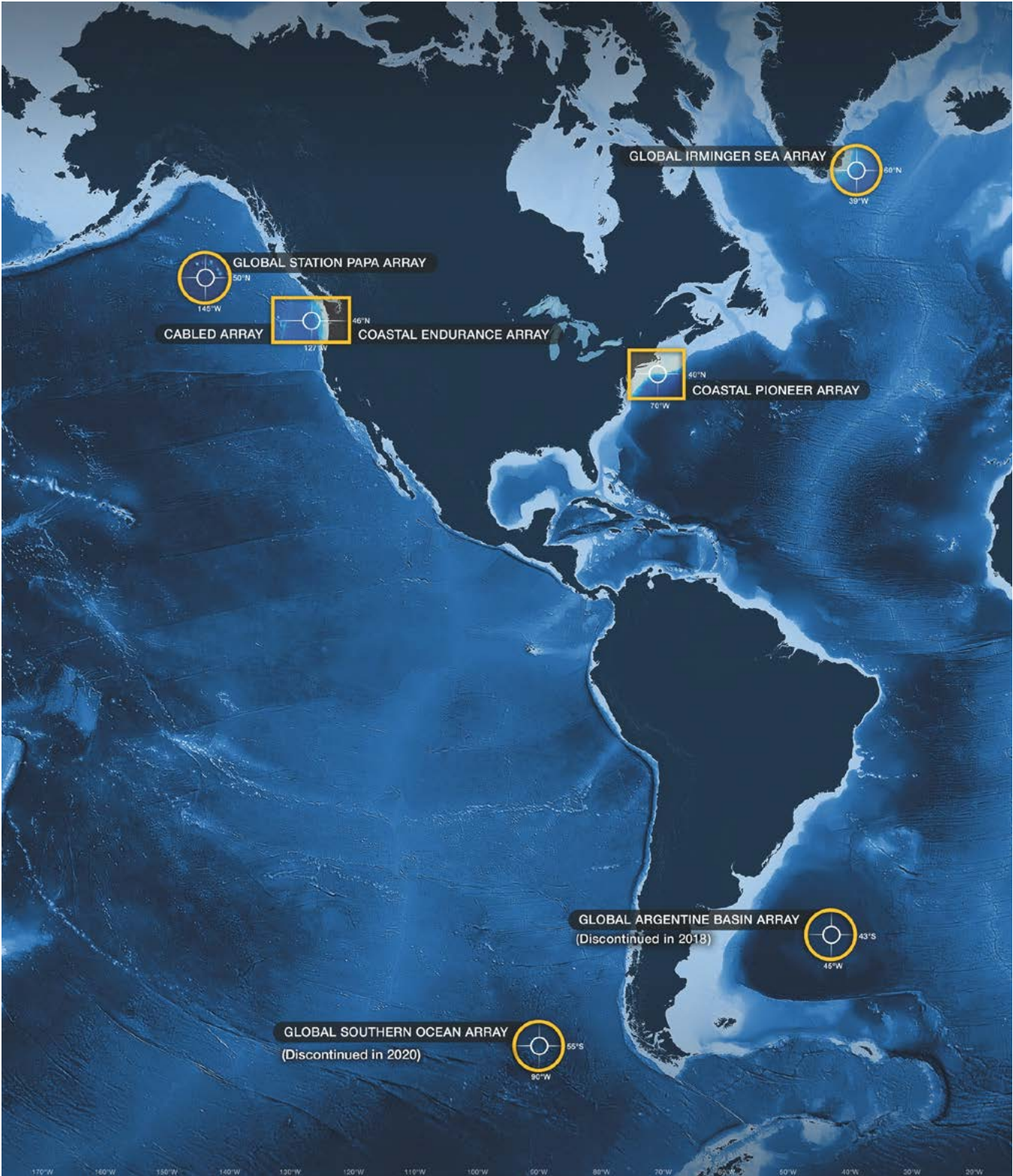
FIGURE 3.1 The OOI consists of five arrays outfitted with some 800 instruments that measure more than 200 different parameters. Credit: Center for Environmental Visualization, University of Washington.
