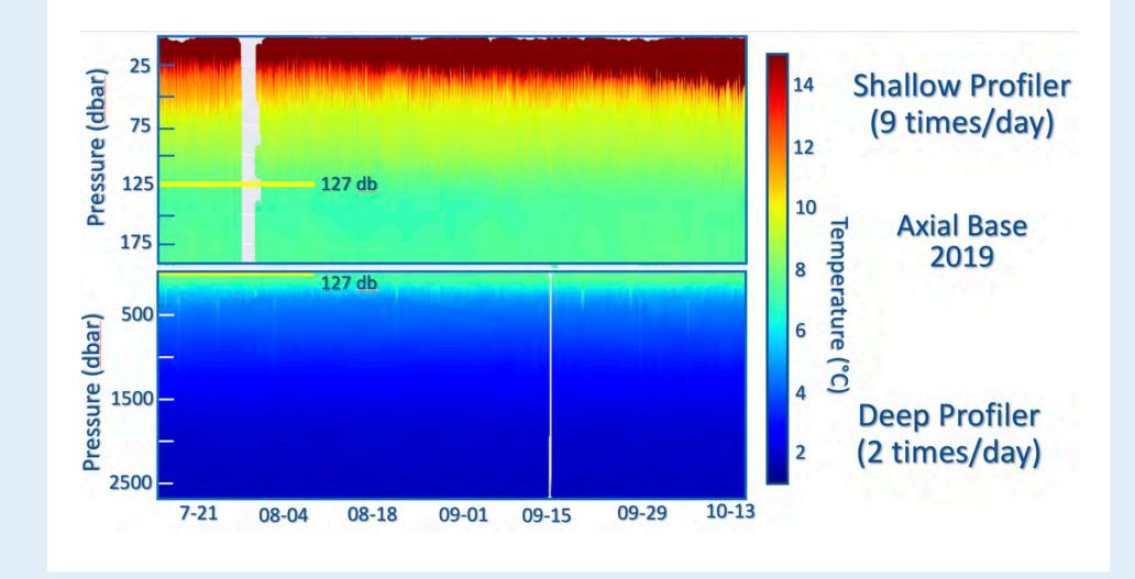
**Axial Base Shallow and Deep Profilers - spanning** 2700 m – 5 m: full water column measurements, 24 instrument suite
