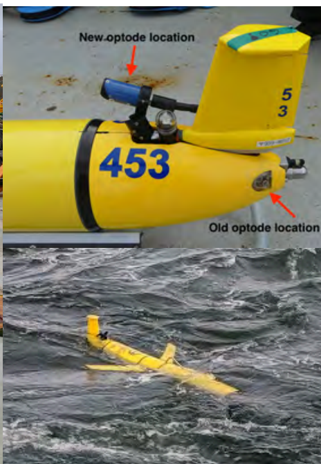
Deployed 2 gliders with air-calibrating oxygen sensors at the OOI Irminger Sea Array in June 2018
