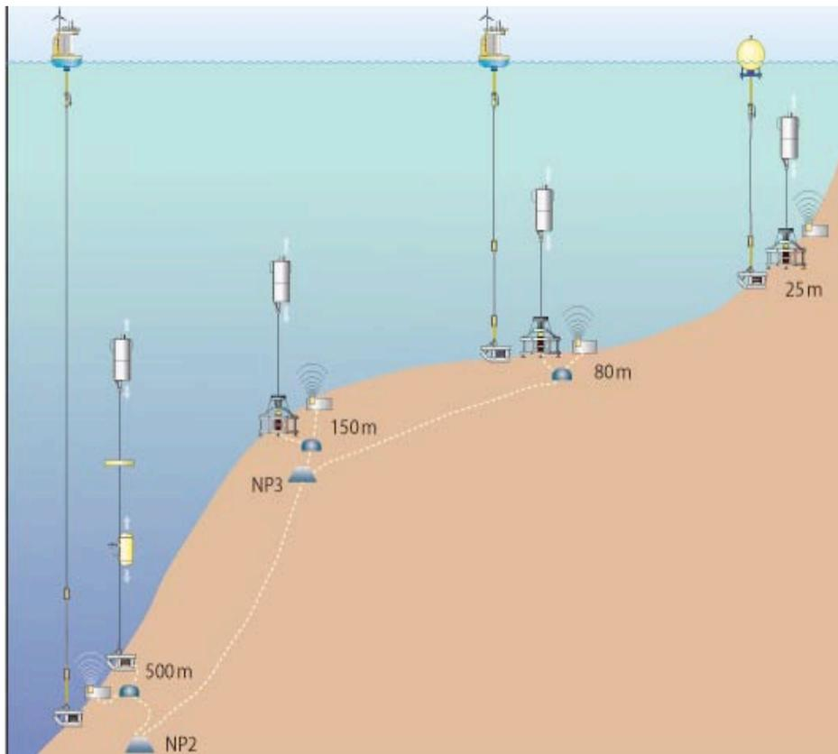
Figure 6. The Oregon line of the Pacific Northwest Endurance Array. Note that the 50-m mooring, which has the lowest priority, is not shown. Attachments to the RSN cable, and the location of surface moorings and subsurface profiler moorings, are drawn in.
