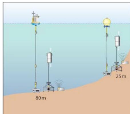
The surface moorings, except at 25 m, will provide the capability to collect surface meteorology and air-sea flux data and will support high-power, high-bandwidth, multidisciplinary science instrumentation in the buoy well and at 5 m beneath the surface. At the 25-m site, the surface buoy will be smaller and hardened against submergence by breaking waves. Fixed sensors will be placed along the mooring lines below surface moorings to provide high-resolution time series.
