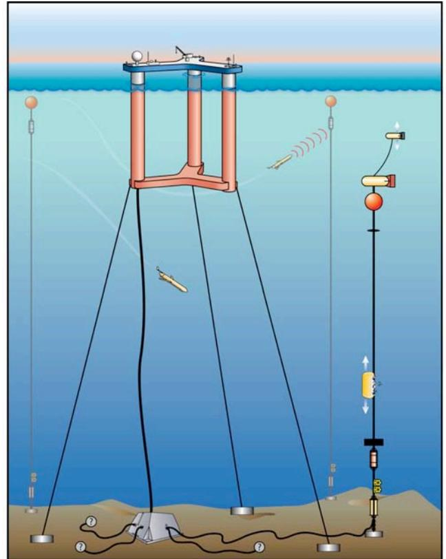
Figure 4. Schematic of the mid-Atlantic global site with the Extended Draft Platform (EDP) installed. As at other global sites, a nearby profiler-equipped subsurface mooring, two flanking subsurface moorings, and gliders will be deployed. An EOM cable to the seafloor from the EDP will provide power to the seafloor and a capable data link back to the surface, supporting seafloor and borehole instrumentation.
