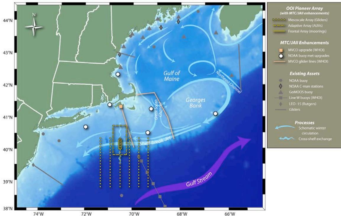
Figure 8. Plan view of the multiscale Pioneer Array in the context of other regional observing elements. A moored array will be centered at the shelf break front and jet south of Cape Cod, MA, AUVs will sample the frontal region near the moored array, and gliders will resolve mesoscale features on the outer shelf and the slope sea between the shelf break front and the Gulf Stream.
