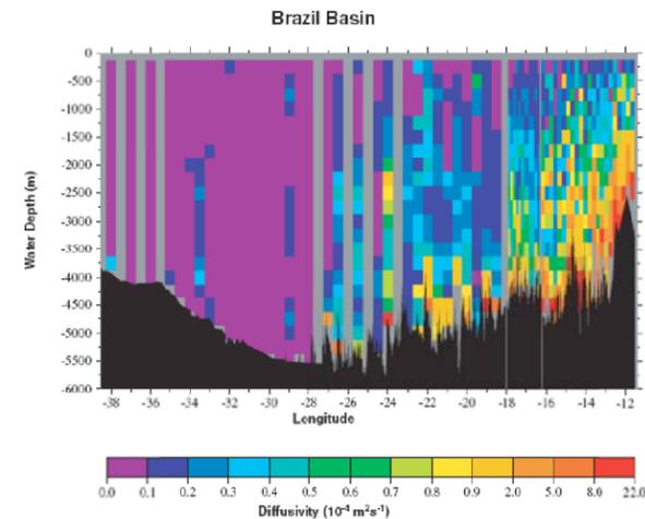
Turbulent diapycnal eddy diffusivity K in the Brazil Basin shows weak mixing (less than  $0.1 \times 10^{-5} \text{ m}^2 \text{ s}^{-1}$ ) over the smooth topography to the west and bottom-elevated mixing ( $K > 10 \times 10^{-5} \text{ m}^2 \text{ s}^{-1}$ ) over the rougher topography of the Mid-Atlantic Ridge to the east (adapted from Mauritzen et al. 2002). Kunze, E. and Llewellyn Smith, S.G. (2004). Oceanography Vol. 17(1): 55-64.
