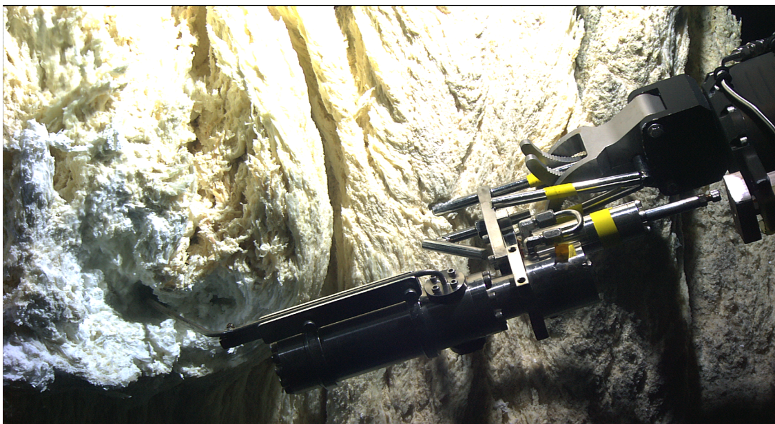
Figure 5. Example of gas-tight fluid sampler acquiring diffuse flow fluids from the Lost City Hydrothermal Field with the robotic vehicle Hercules.
