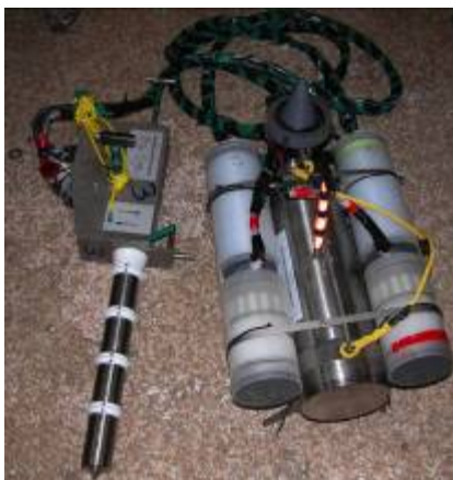
Figure 7. Two loaded Osmo (OSMOI) Sampler canisters are attached to a data logger and microbial incubator awaiting deployment in a black smoker chimney on the Endeavour Segment of the Juan de Fuca Ridge. In this example, the inlets are housed within the barrel of the incubator.
